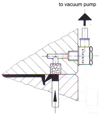
Fig. 7: Venting diagram (Bawema)
