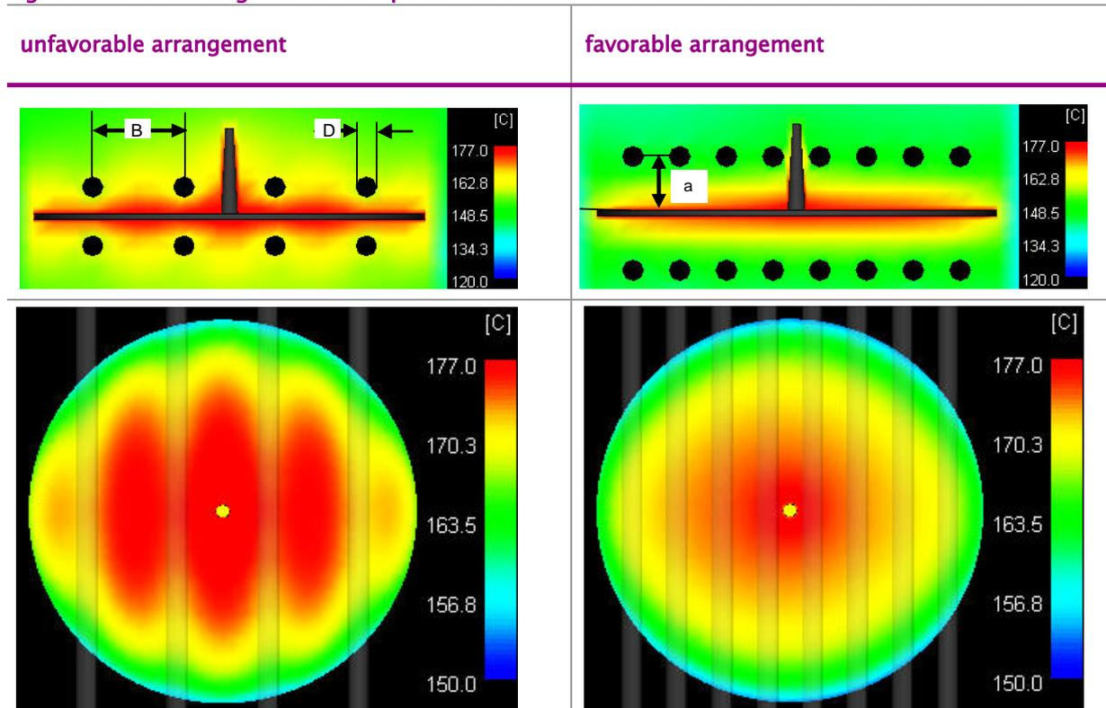
Example of an even sheet: wall thickness = 2.5 mm, tool temp.=180°C, compound temperature = 340°C
