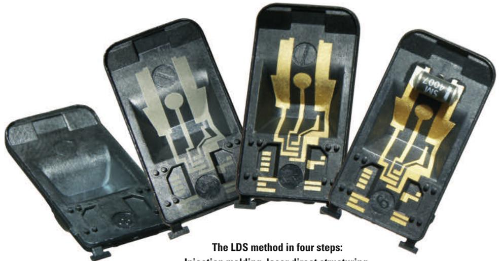
The LDS method in four steps: Injection molding, laser direct structuring, metallization, mounting (photo: LPKF)
