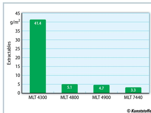
**Fig. 4.** The soluble extractables at 23 °C with FAM-B laboratory fuel as per VWTL52712 in the case of 8x1 mm tubes show that the new MLT product range features significantly less extractables (source: Evonik)
