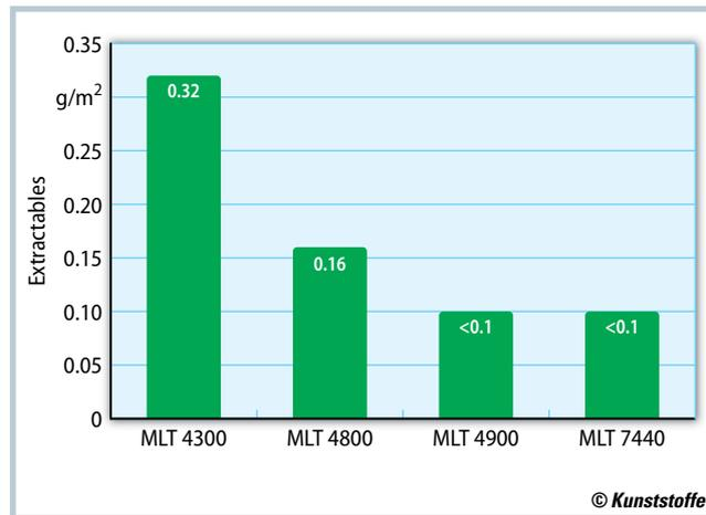
**Fig. 5.** Presentation of the insoluble extractables at 23 °C with FAM B laboratory fuel as per VW TL 52712 at 8x1 mm tubes. The insoluble extract concentration lies within the measurement accuracy range of the test method
