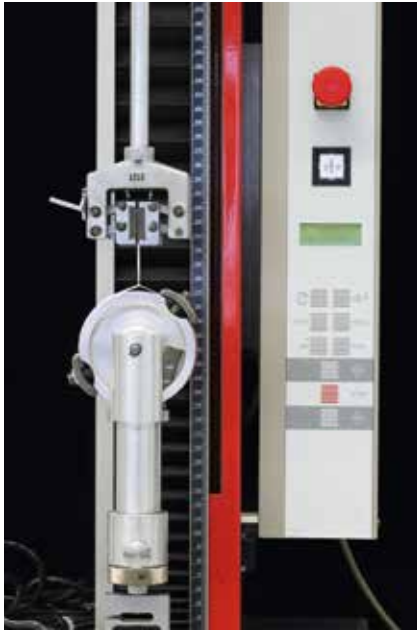
Fig. 1. Set-up of a roll peeling test for determining the layer adhesion of a multilayer plastic tube with a tensile testing machine
