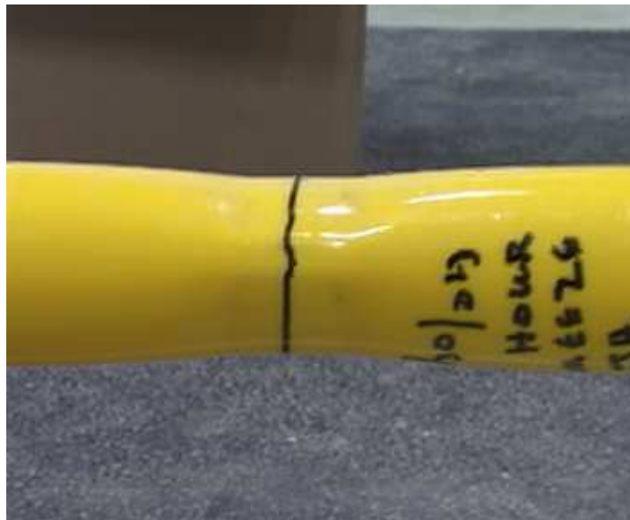
Figure 17: Completed squeeze-off on PA12
