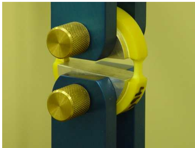
Figure 3. Apparent Tensile strength determination testing for PA12 pipe specimens
