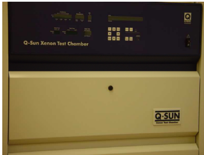
Figure 14: Q-Sun Xenon Test Chamber
