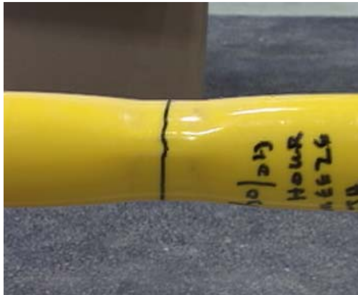
Figure 10: Completed squeeze-off on PA12 pipe
