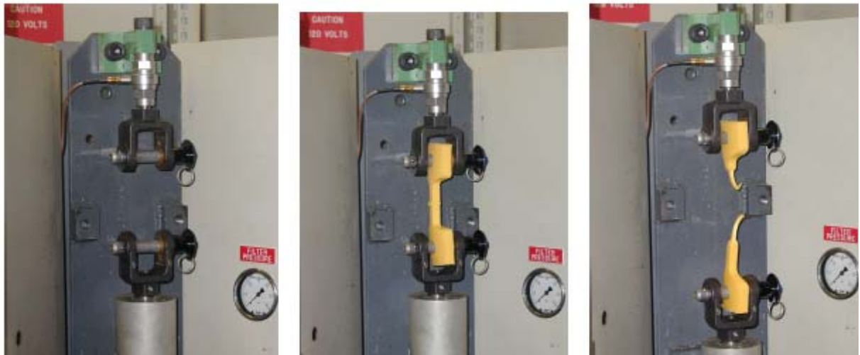
Figure 4: Typical McSnapper™ test set-up and testing progression of a typical PA12 test specimens at an average speed of 6 in/s.
