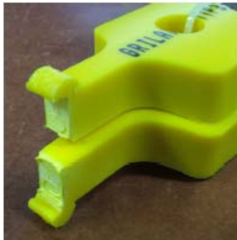
Figure 5: Illustration of the fracture surface of a PA12 joint which did not satisfy the visual criteria for an acceptable joint
