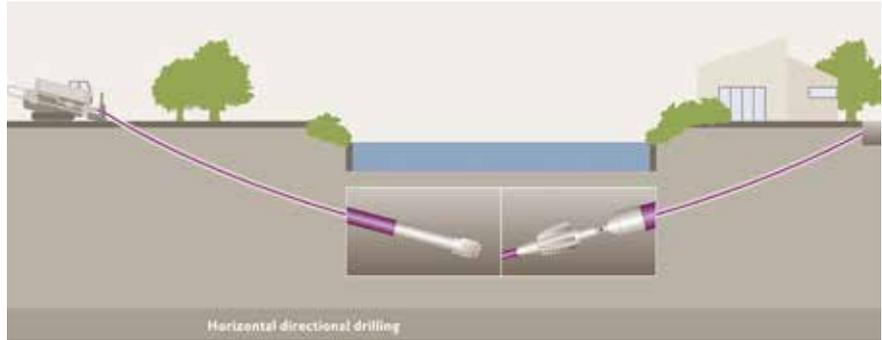
**Fig. 4.** Directional drilling is just one of several methods for trenchless laying of underground pipes. PA12 pipes must meet the various mechanical requirements imposed
