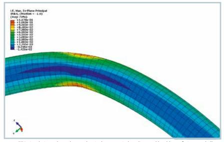
**Fig. 5.** FEA simulations show the mechanical stresses in bending and buckling of pipes and allow reliable predictions and recommendations to be made (shown here the buckling of a pipe under bending stress)
