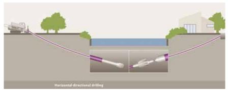
Fig. 4. Directional drilling is just one of several methods for trenchless laying of underground pipes. PA12 pipes must meet the various mechanical requirements imposed
