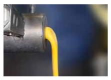
**Fig. 1.** Top: Schematic diagram of the impact of pipe dimension on horizontal extrusion (left: high viscosity; right: low viscosity). Center: Extrusion of material with high viscosity and/or melt strength. Bottom: Extrusion of material with low viscosity and/or melt strength
