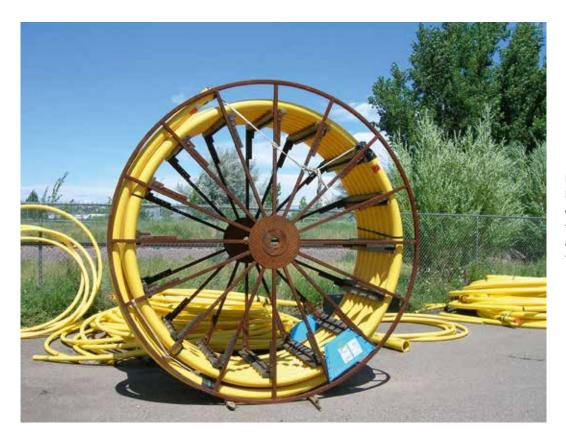
PA12 piping up to 200 m long can be rolled up. In contrast, trucks can only transport steel pipes with a maximum length of 18 m (figures: Evonik Industries)
