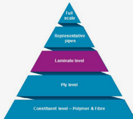
Testing pyramid from constituent materials to the TCP system as shown in DNV-ST-F119.
