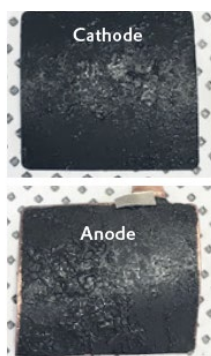
Photographs of the opened cell after formation: Composite gel polymer electrolyte is clearly visible
