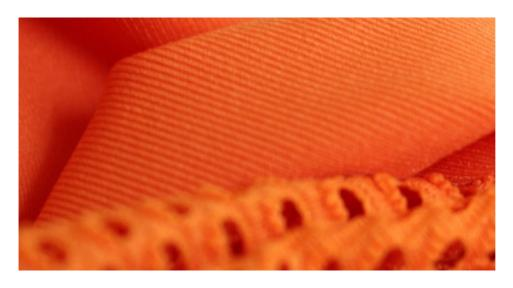
**Photo caption:** Fabrics made from the bio polyamide fibers EVO® based on VESTAMID® Terra (Source:Fulgar).
