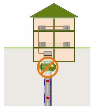
Caption: Direct heat exchanger technology using VESTAMID® polyamide 12 tubes improves the efficiency of geothermal energy production by a further 10 percent.
