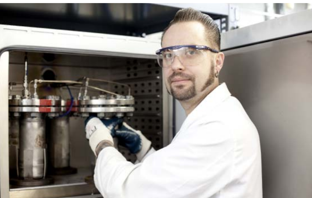
Chemical laboratory technician Karsten Hinnah simulates prolonged stress from high temperatures in the furnace.
