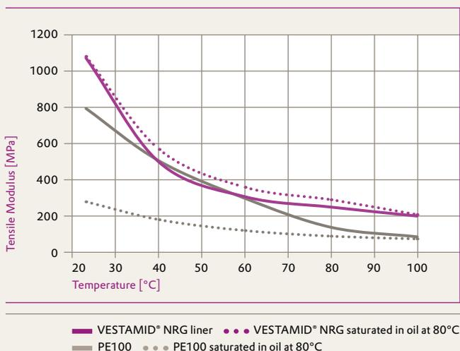
9 – Significant reduced mass swelling of VESTAMID® NRG 3000 series allows safe operations and avoids buckling
